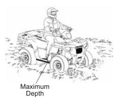
**NOTICE:** Major engine damage can result if the vehicle is not thoroughly inspected after operation in water. Perform the services outlined in the maintenance chart. See page 62. The following areas need special attention: engine oil, transmission oil, demand drive fluid, rear gearcase oil, and all grease fittings.
